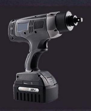
The LTB's industrial-strength gear box is driven by a brushless DC motor connected to a non-impacting gearbox to deliver torque faster, smoother and more reliably than manual clicker wrenches, impact wrenches and other tightening tools.
