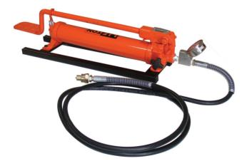
Lifton manual foot pump kit consist of 3 meters long high pressure hose assembly fixed with quick male relese coupler at one end. Also supplied with 64mm dial glycerine filled dual scale, 0-700 bar/0-10000 psi pressure gauge fixed on a gauge mounting block.
